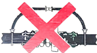
Incorrect Method - Excess Slack
